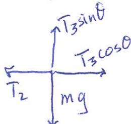
$$\text{vertical: } T_3 \sin\theta = mg \quad T_3 = \frac{mg}{\sin\theta} = \frac{(0.25\text{ kg})(9.8\text{ m/s}^2)}{\sin 46^\circ} = 3.4\text{ N}$$
