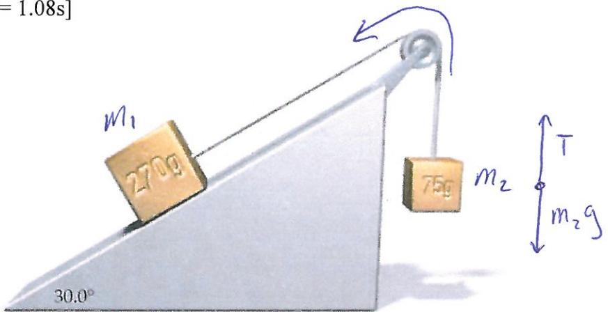
Forces on hanging blocks: Tension of rope, gravity
