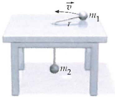
This same string is holding up  $m_2$ , so balancing vertical forces on  $m_2$  (no motion of  $m_2$ ):
