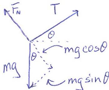
$$\begin{aligned} \text{along ramp: } & m_1 g \sin \theta - T = m_1 a && (\text{down ramp is positive}) \\ \perp \text{to ramp: } & F_N - m_1 g \cos \theta = 0 \end{aligned}$$
