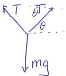
Break  $\vec{T}$  into horizontal and vertical components
