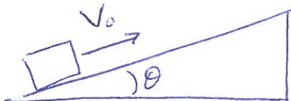
First find the acceleration (negative) of the box using Newton's second law, then use  $2a\Delta x = V_f^2 - V_0^2$  to get distance up the ramp.
