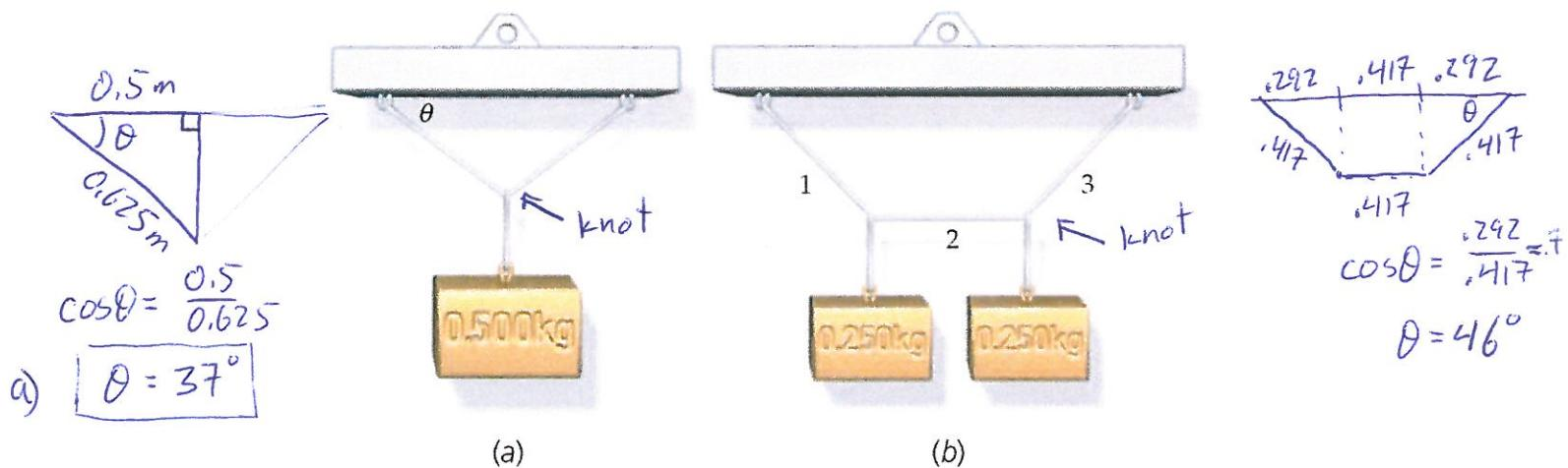
b) Find the tension in the string by applying  $\sum \vec{F} = m\vec{a}$  to the knot where the strings are connected.
